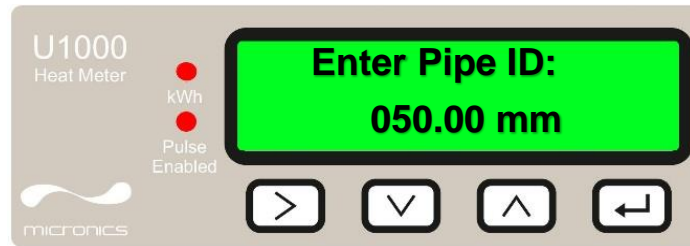
Figure 10 Enter Pipe ID Screen (Metric)
